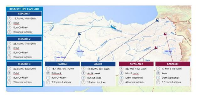
I - installed capacity and 2021 annual generation; R - river; T - type of the HPP (with reservoir or run-of-the-Legend: river); E - # of turbines + type;
